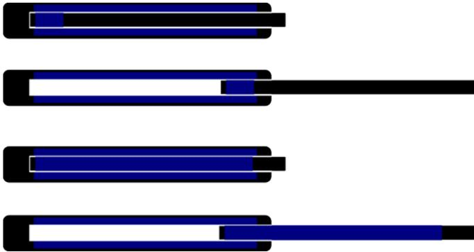
The top two diagrams show a constant-force EM ram, the lower two show a variable force ram. The blue areas show the locations of the superconducting coils. In the lower example the force decreases as the ram extends because there is steadily decreasing overlap between the two sets of blue coils as the ram moves.
